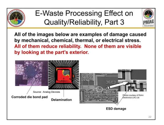
These images are all of electronic parts that have either failed, or are likely to fail soon. The handling, stacking, removal, and refurbishment of electronic parts and assemblies, if not closely controlled, will cause damage like this. None of the damage is readily visible on the outside of the package. Parts can be damaged mechanically, chemically, thermally, and electrically.
