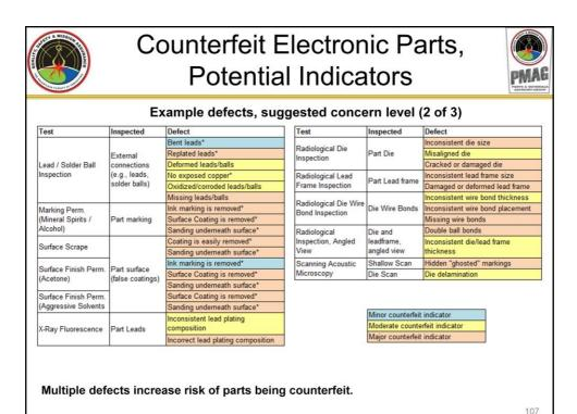
Here is the second slide on counterfeit part indicators. These indicators in concern levels were generated from information in IDEA-STD-1010B, GIDEP Alerts, and inputs from various DoD representatives. This should not be assumed to include all counterfeit indicators for electronic parts.
