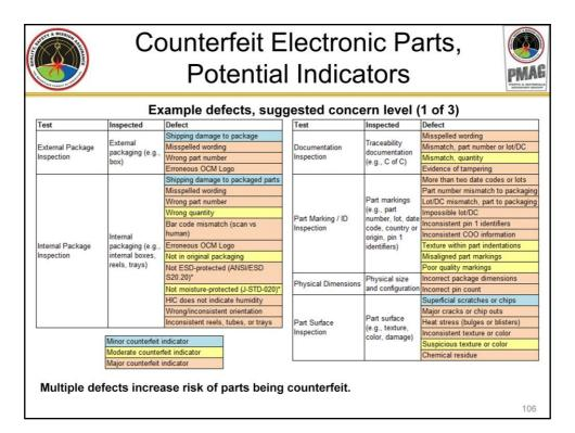
The information in the next three slides provides many potential indicators of a counterfeit electronic part, along with guidance on the importance of the indicator. Defects in orange shading are strong evidence of counterfeiting. All of the other defects may also indicate the part is counterfeit, but the confidence is reduced. A minor indicator for counterfeiting might still be a moderate or major quality concern.
