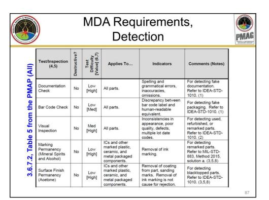
MDA's PMAP Table 5 requires specific part-level inspections and tests for all parts bought from unauthorized suppliers. Those required inspections and tests are called authenticity tests, and they are listed on the next three slides. They include:
