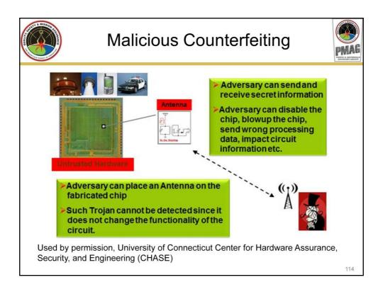
This slide from the University of Connecticut's Center for Hardware Assurance, Security, and Engineering, or CHASE (pronounced 'chase'), shows how a critical part can be modified slightly, leaving very little visual evidence of the change. The part could then be called upon by our enemy to:
