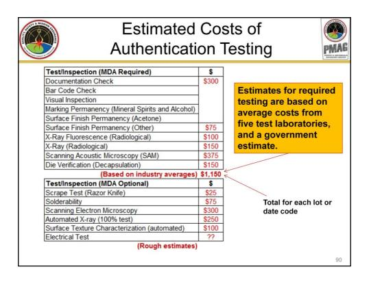
How much does it cost to validate whether a shipment of electronic parts is authentic? MDA queried five industry test laboratories, as well as a government test facility. While the estimates varied widely, the average cost of performing all of MDA's required inspections and tests should be approximately \$1,150 per lot or date code. These estimates assumed the part was a medium complexity integrated circuit, although the cost did not change significantly for part complexity or lot size.
