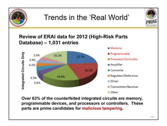
Of over 850 suspect counterfeit integrated circuits reported to ERAI in 2012, over 63 percent of them were either memory circuits, programmable devices, processors, or controllers. This is significant because these part types might provide the most value if an enemy wished to insert malicious code or circuitry into the part. These parts are the most likely to store critical system information, or be able to cause complete system failure if so desired.
