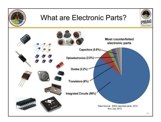
There are many different types of electronic parts, in many shapes and sizes. Prices range from less than a penny to thousands of dollars each. Some parts are readily available from trusted sources, and others are very difficult to find. Electronic parts include integrated circuits, or IC's, transistors, diodes, resistors, capacitors, inductors, relays, connectors, displays, and many other part types.
