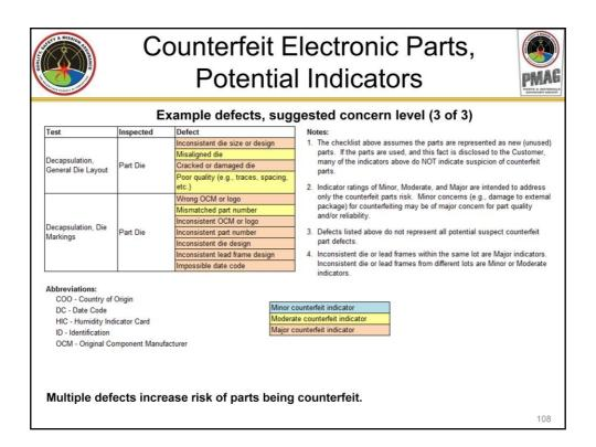
This is the final slide of indicators. Keep in mind that this assumes that the customer has requested new parts. There are many refurbished, or used, parts available in the open market. If they are not being sold as new parts they are not counterfeit, unless the parts have been misrepresented in other ways, such as wrong die, date code, temperature range, and so on.
