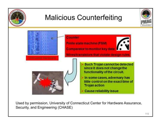
This additional slide from CHASE indicates that control over the 'destruct state' is likely to be limited. However, the part might be designed to monitor key events and data transfers, which increases the chances of shutting the system down during a critical activity.
