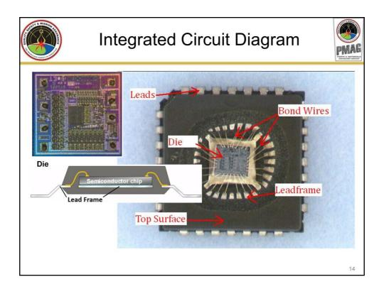
As mentioned on the previous slide, integrated circuits are made of tiny electronic parts, both passive and active, that are connected together to make a circuit that performs a specific function. The tiny parts are designed and produced in a very small package called a die. The outputs on the die are attached to a lead frame by very tiny wires, called bond wires. The lead frame includes the part's external connections, usually called pins or leads.
