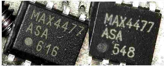
Part marking is blurred compared to authentic part
