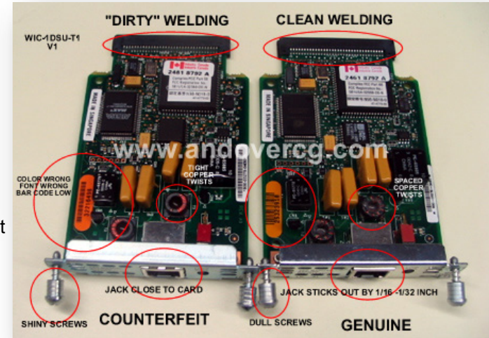
Marking slightly different on counterfeit part
