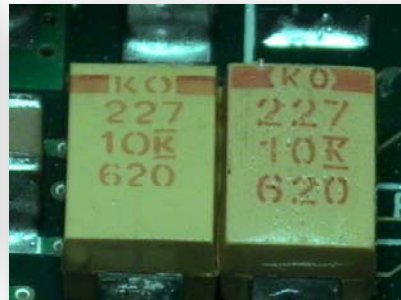
Marking slightly different on counterfeit part
