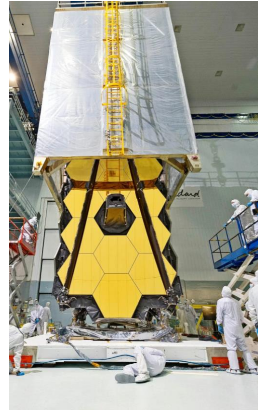
James Webb Space Telescope being prepared for vibration testing. Photo credit: NASA/Chris Gunn
