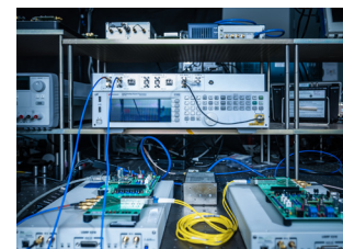
The digital propagation delay emulator (center rack, top) uniquely enables signal true time delays and Doppler shifts commensurate with the low-Earth to cis-lunar orbits. This technology is based on Aerospace proprietary technology.
