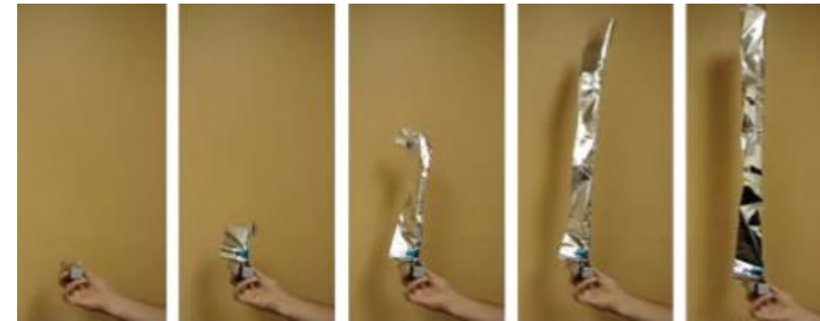
Deployment progression for 3U CubeSat RODEO [2]
