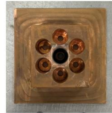
Figure 1. Image of copper thruster array with slots for 7 anodes
