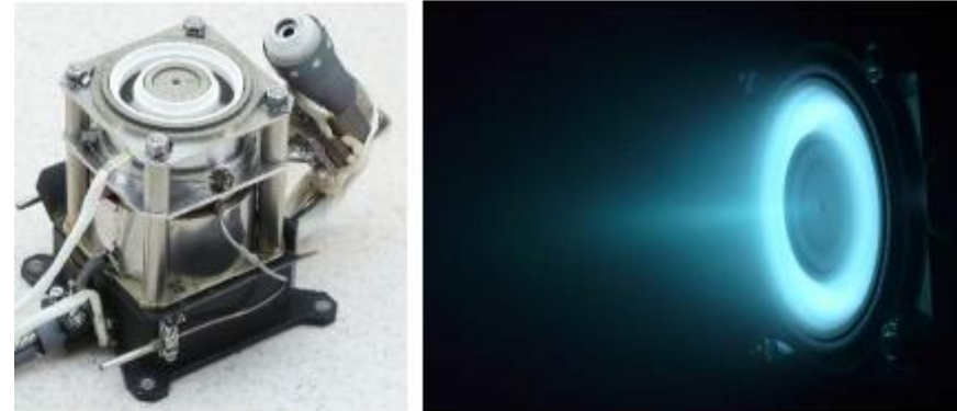
PlaS-34 thruster after manufacturing and during operation
