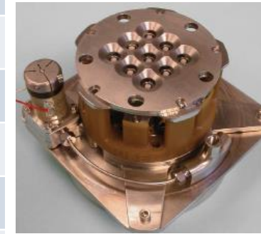
Busek's BET-1mN electropray thruster
