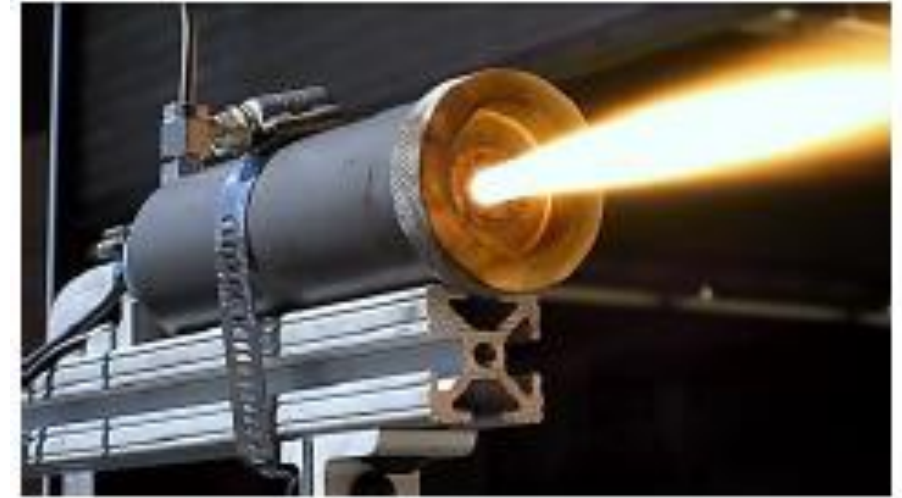
Figure 1. Static Hot-fire Test of Prototype 25-N Thruster Unit.
