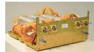
SkySat-3 HPGP flight system. Multiple 1N systems installed.
