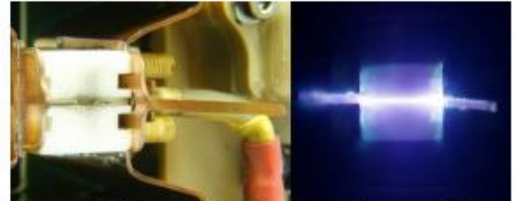
Figure 18. Thruster equipped with flared (22.5°) narrow electrodes (0.5 mm×1.0 mm×20 mm).
