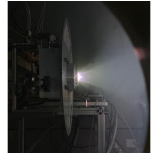
Maxwell firing on water propellant, above, and operating in vacuum chambers (two images below) [11]
