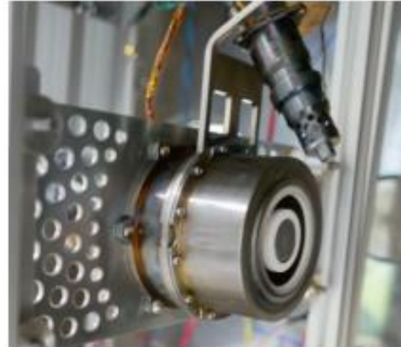
Fig. 2. 5-mN Hall-Effect Thruster as preliminary version of HET-2
