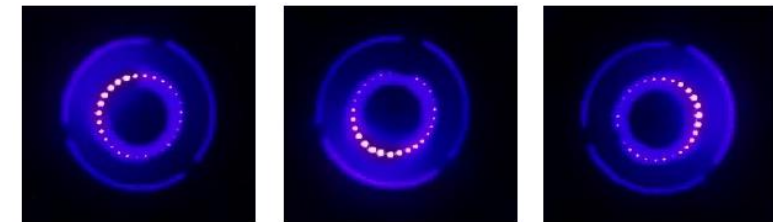
Thrust vectoring capability of the ENPULSION NANO AR 3
