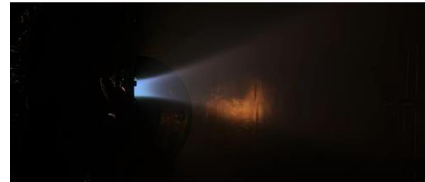
Fig. 6 Low-voltage ET mode with D = 5 mm, 40 A, 0.48 T, and 15 mg/s.
