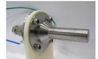
Figure 5. Picture of Rafael's R-800 Heaterless Cathode (ARC-2A)
