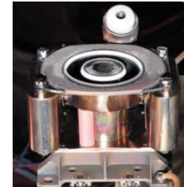
PlaS-40 thruster after 200 hrs operation time
