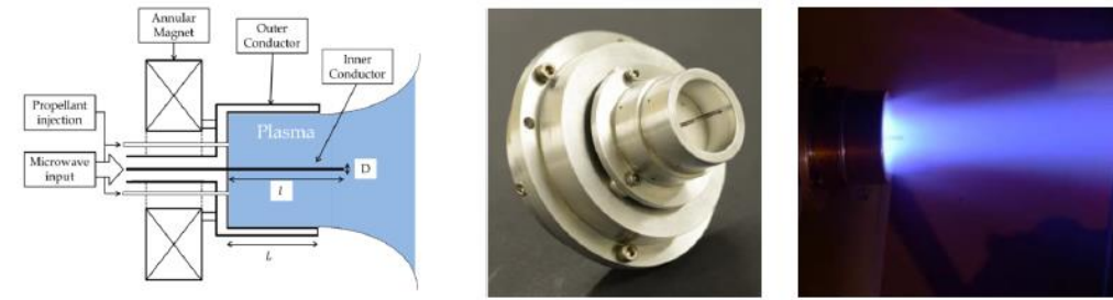
Fig. 1 (left) ECRA thruster geometry, (center) picture of a 30 W ECRA thruster, (right) operating ECRA thruster
