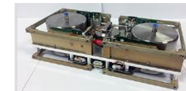
GomX-4B's cold-gas thruster system takes up two half-cubesat units at one side of the nanosatellite, with two spherical titanium tanks filled with liquid butane. It has four 1 mN thrusters, typically to be fired in pairs while keeping one set in reserve. Photo is courtesy of Nanospace.
