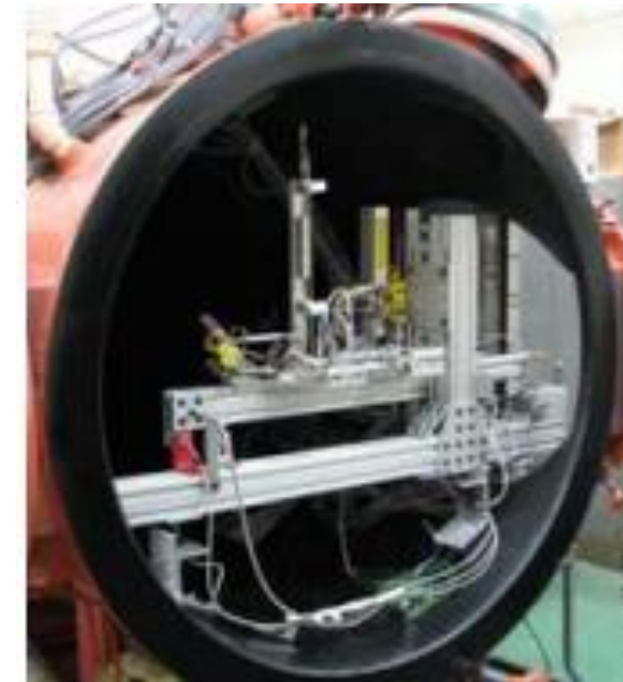
Thruster installed on JPL milli-newton thrust stand
