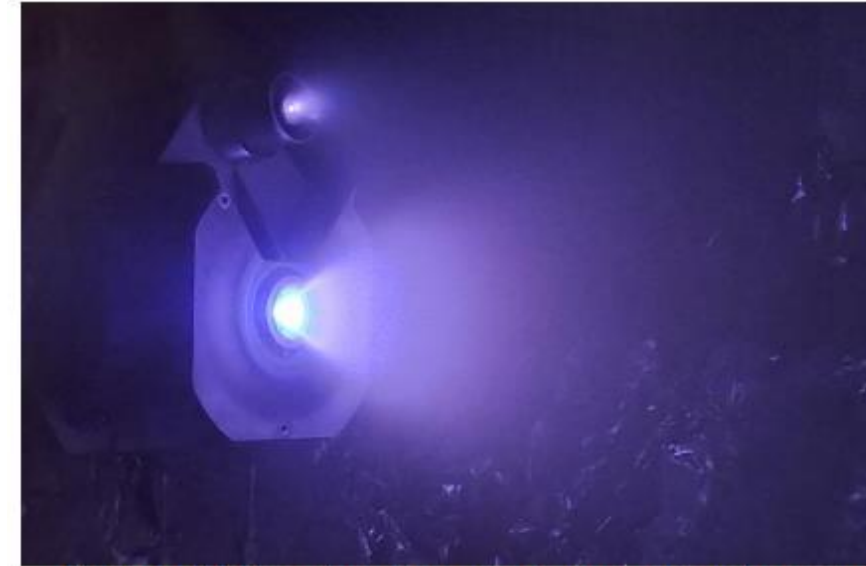
Fig. 11. HEMPT operating with krypton during coupling test campaign
