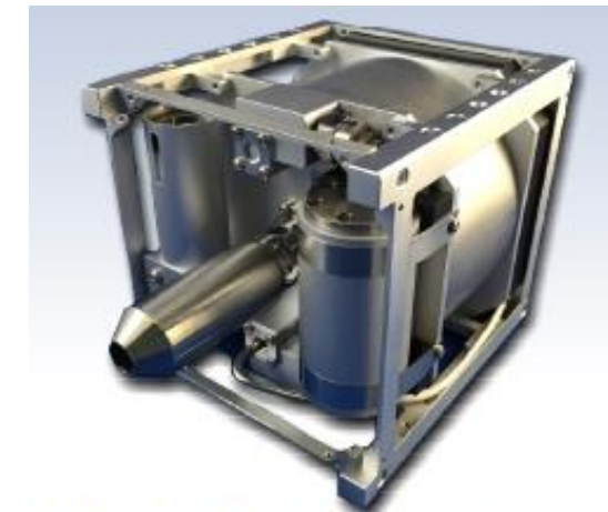
1U CubeSat Green Propulsion System
