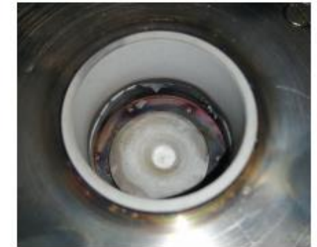
Fig. 4 Eroded central ceramic
