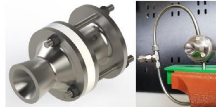
Figure 9. CAD of the arcjet prototype (left) and arcjet experimental prototype (right).
