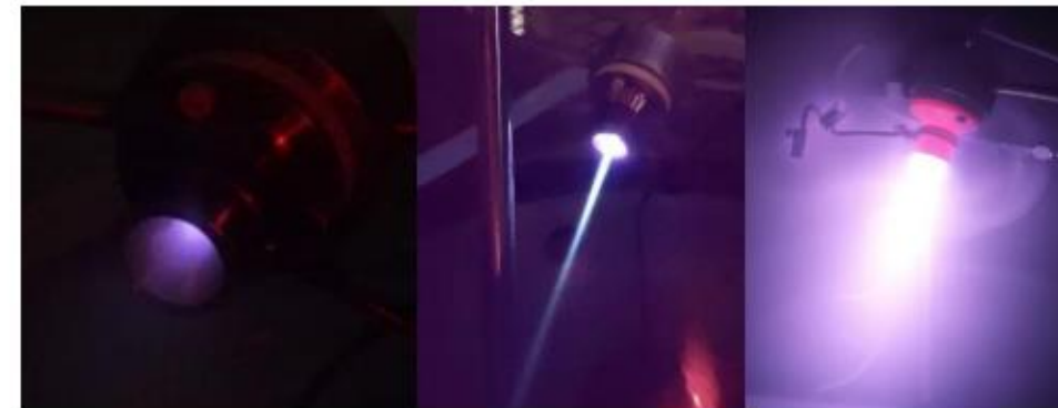
Figure 10. LaSE arcjet operating in three different discharge regimes.
