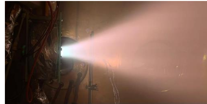
Fig. 5 Stable operation of ET mode with D = 0 mm, 50 A, 0.48 T, and 21 mg/s.
