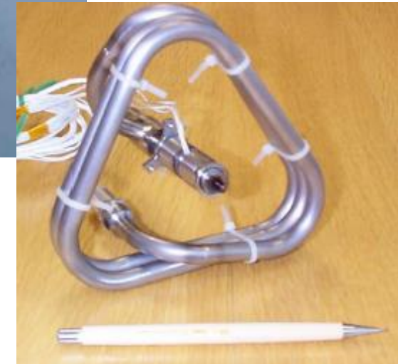
SNAP-1 vehicle, with butane propulsion system
