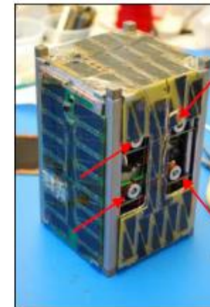
Thrusters, incorporated into BRICSat-P, a 1.5U CubeSat with 4X GWU micro-CAT thrusters
