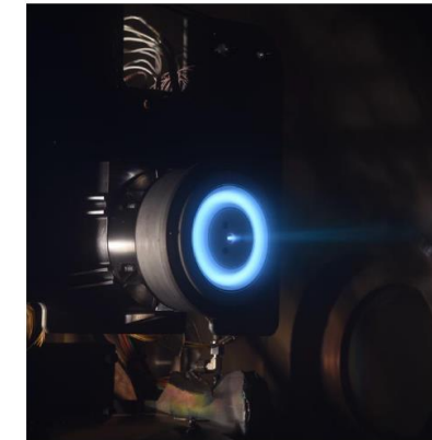
Figure 3. NGHT-1X firing in NASA's VF-8 facility.
