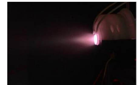
Photo of the thruster firing inside Phase Four's chamber.
