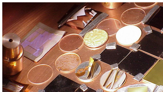
These materials were exposed to laboratory-simulated space radiation for a period of 14 years.
