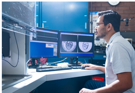
A scientist operating the scanning acoustic microscope.
