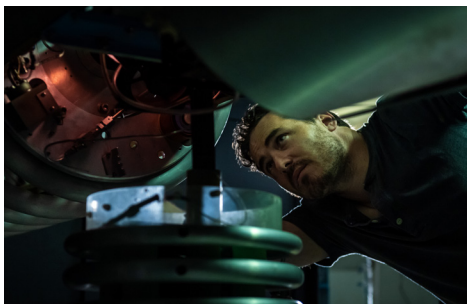
Our scientists use this proton accelerator to simulate proton radiation from space, which is one of the main causes of solar cell failure.
