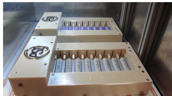
COTS Li-ion cells in test fixtures.
