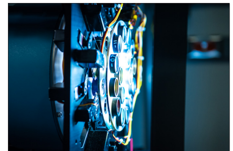
The custom Xe-lamp based solar simulator is highly tunable for measuring all advanced space solar cell technologies.
