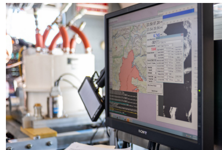
MAHI (left) is a midwave infrared scanner capable of 640 bands of spectral resolution. During the Creek Fire of 2020, it was used to measure toxic gases during a series of flyovers.
