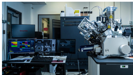
The plasma focused ion beam is a unique capability that can image, cut, manipulate, weld, and analyze microelectronic devices all in one.
