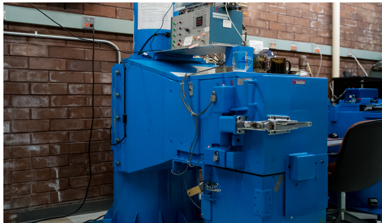
Aerospace's 7000 Ci Co-60 irradiator tests samples to determine how they would respond to the space environment.
