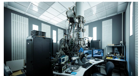
The transmission electron microscope transmits a beam of electrons through a sample to create an image at incredibly high resolution.
