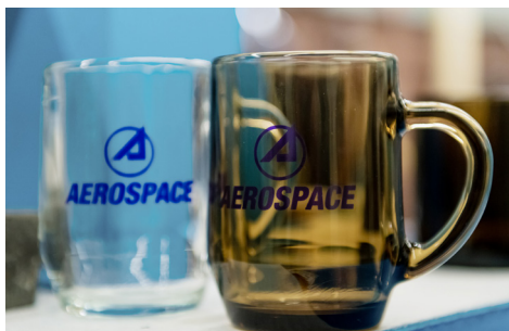
The mug on the right was placed inside the Co-60 irradiator, and demonstrates the effects of radiation on glass.
