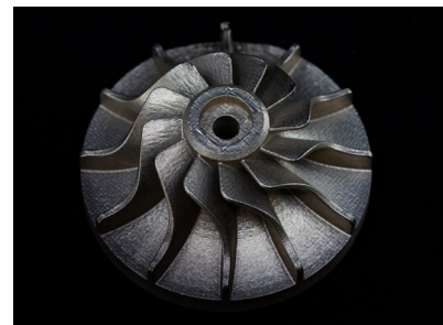
Additive manufacturing enables the production of geometrically complex parts as monolithic pieces, increasing manufacturing efficiency while reducing costs and lead times.
