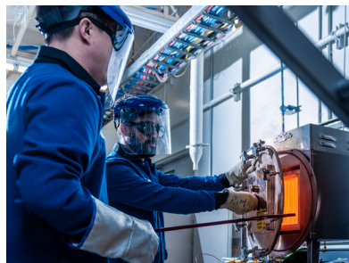
Aerospace scientists prepare to quench metal samples during the heat treatment of Ni-based superalloys.
