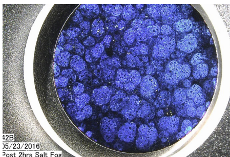
A salt fog test performed on a mirror resulted in distinct blue, cloud-like shapes, which are chemical corruptions on the mirror surface caused by the salt.
