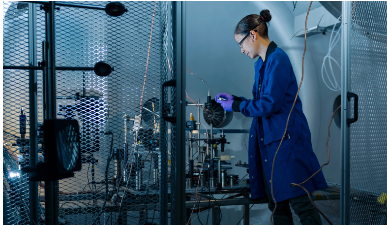
Senior Scientist Andrea Hsu examines an optical component for the torsional thrust stand, which is used to measure very small amounts of force in a vacuum environment.
