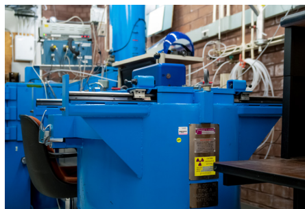
Some devices actually have more trouble with a low dose of radiation, and this low dose-rate Co-60 irradiator is specifically for testing those types of devices.
