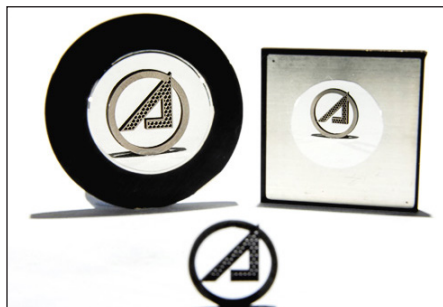
Comparison of a curved and a flat mirror: the object being imaged, at bottom, is a 3-D printed Inconel® Aerospace logo. The reflected image in the curved mirror at left appears magnified compared to the flat mirror on the right.
