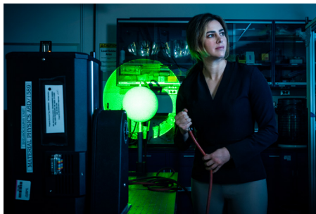
Shearography is used to inspect a composite overwrapped pressure vessel, revealing weak spots due to damage.
