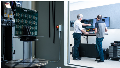
Our scientists use X-ray CT scanners to peer deep inside space systems and their components in search of flaws.
