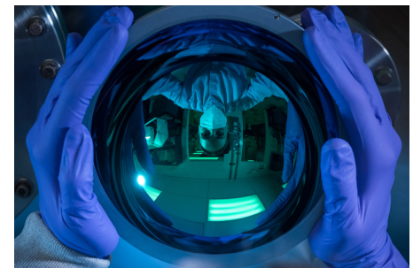
Example of an advanced optical coating deposited on a curved substrate.
