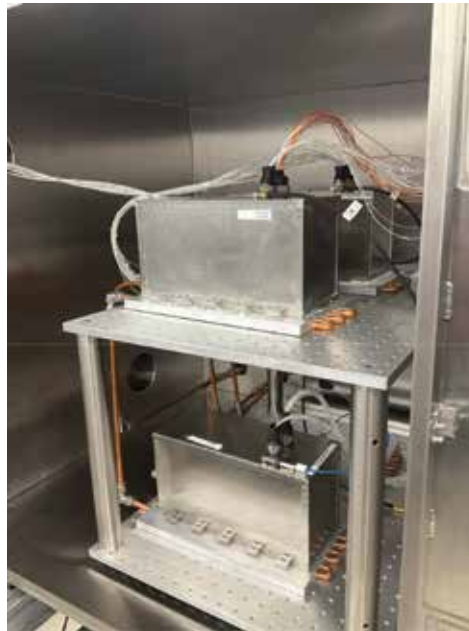
Left: The thermovac chamber. Right: Example setup of using a GPS RAFS in the thermovac chamber.
