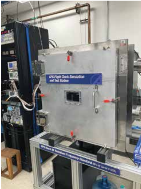
Left: The thermovac chamber. Right: Example setup of using a GPS RAFS in the thermovac chamber.
