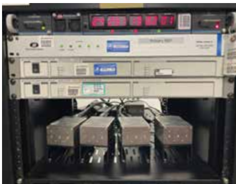
Left: The PRS10s that constitute the ensemble. Right: Block diagram of testbed config. Clocks are input to the multimeasurement system with the clock called "Evil Kevin," the recipient of the emulated noise types.
