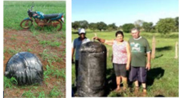
Figure 12. Recovered composite overwrapped pressure vessels (COPVs). The left photo shows debris from the Centaur stage of an Atlas V booster, and the right photo shows the SpaceX Falcon 9 stage.
