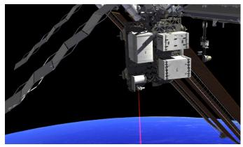
Optical Payload for Lasercomm Science (OPALS) was developed at JPL and tested on the ISS in 2014 to demonstrate laser communications between spacecraft and ground stations. Credit: NASA.
