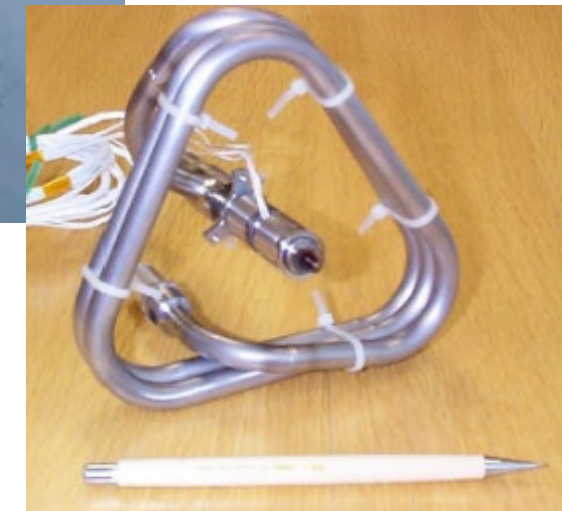
SNAP-1 vehicle, with butane propulsion system
