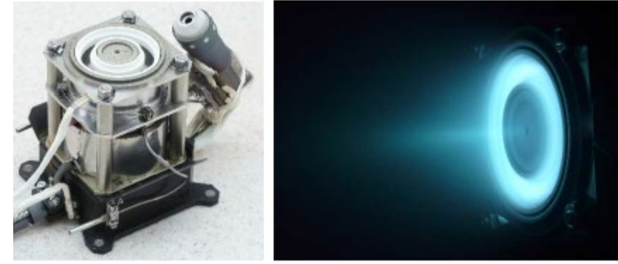
PlaS-34 thruster after manufacturing and during operation
