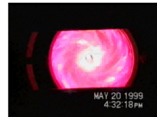
Vortex flow combustion seen through a plexiglass fuel grain (for flowfield demonstration)
