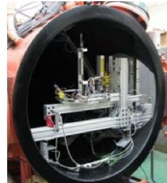
Thruster installed on JPL milli-newton thrust stand
