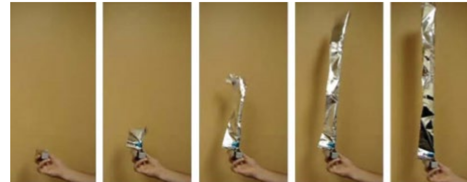
Deployment progression for 3U CubeSat RODEO [2]
