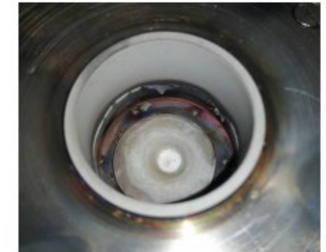
Fig. 4 Eroded central ceramic
