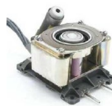
PlaS-40 thruster after manufacturing and during operation
