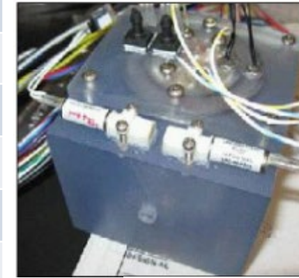
Aerospace's AC7 additively manufactured steam propulsion unit.
