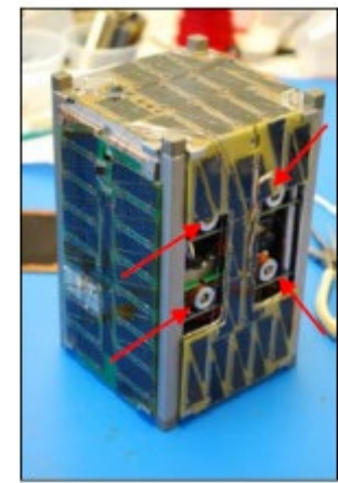
Thrusters, incorporated into BRICSat-P, a 1.5U CubeSat with 4X GWU micro-CAT thrusters
