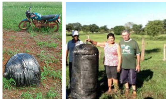
Figure 8. Recovered composite overwrapped pressure vessels, or COPVs. The left photo shows debris from Centaur stage of Atlas V booster, and the SpaceX Falcon 9 Stage can be seen in the right photo.
