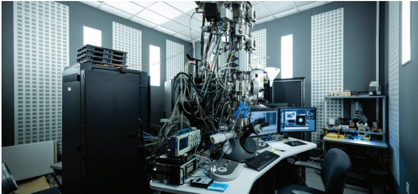
The Transmission Electron Microscope can perform atomic-resolution imaging of state-of-the-art semiconductor devices.
