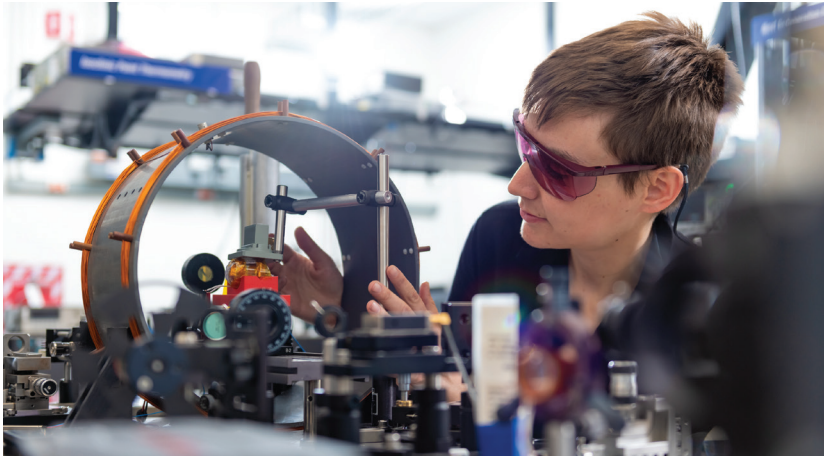
Dr. Daniele Monahan investigates the microwave interrogation on a next-generation atomic clock testbed.
