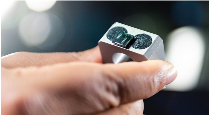
A photonic integrated circuit designed and built by Aerospace.
