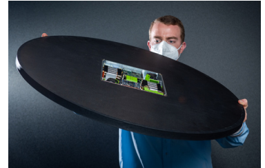
DiskSat is a plate-shaped satellite, 1 m in diameter, 2.5 cm thick.
