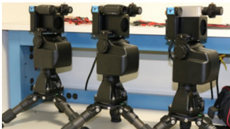
The small form factor of the mini-beacon makes it ultra-portable for operation at a single wavelength in the shortwave infrared band.
