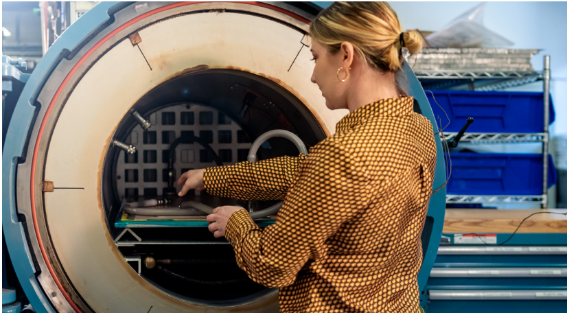
The composites used as a substrate for the optics are made in an autoclave, which controls the temperature, pressure, and cure time for composite fabrication.
