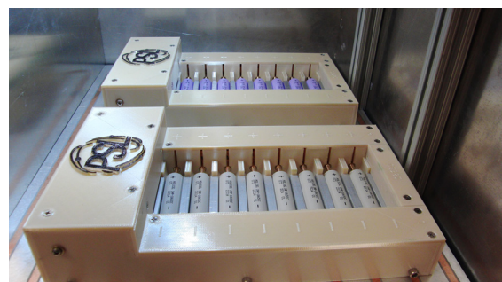
COTS Li-ion cells in test fixtures.
