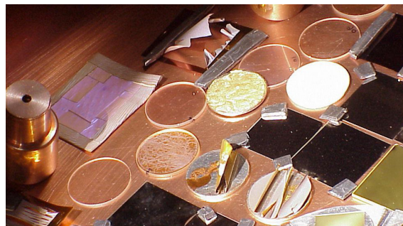
These materials were exposed to laboratory-simulated space radiation for a period of 14 years.
