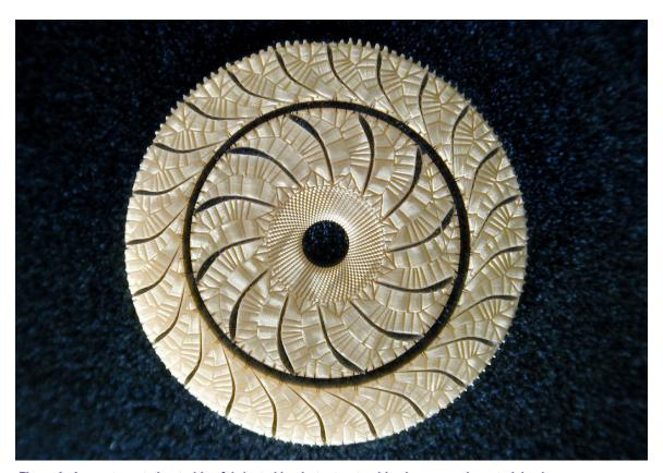
Figure 9: A counter-rotating turbine fabricated in photostructurable glass ceramic material using a novel laser machining technique.
