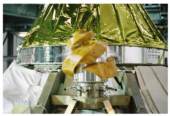
Figure 3: JAXA art mission DESPATCH attached as a secondary payload to the Hayabusa-2 spacecraft prior to launch. (Credit: JAXA, used with permission)<sup>10</sup>
