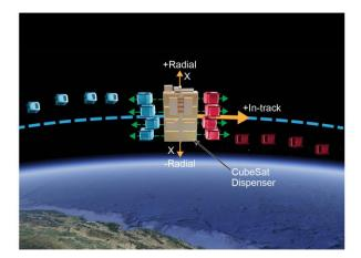
Figure 2: Note the "string of pearls" above and below dispenser altitude achieved by deploying pairs of CubeSats in the +/- in-track direction. Deploying along a radial and cross-track would lead to "bunching," which causes confusion, cross-tagging, and misidentification.
