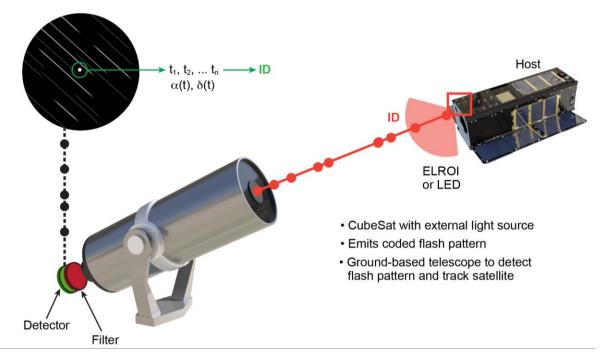
Figure 4: Displays a scheme with a CubeSat outfitted with an external light source, one with a distinct flash pattern, being detected and identified by a ground-based optical telescope.
