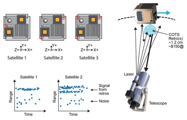
Figure 6: Displays a scheme to outfit CubeSats with small COTS retroreflectors. By varying the number of retros on the face of a CubeSat, different returns are observed when illuminated with a ground-based laser and observed with a co-located telescope.
