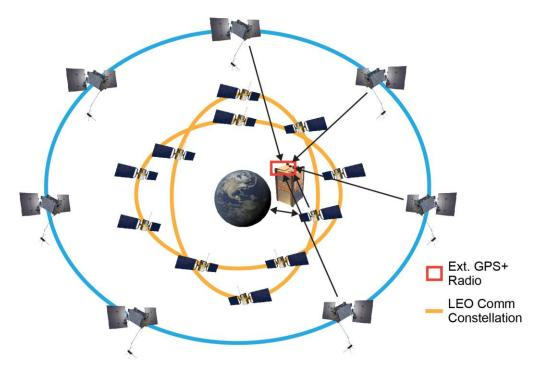
Figure 3: The PNT-derived coordinates of the CubeSat ((x,y,z,t) + ID) might be radioed down via a low-bandwidth LEO communications constellation. (Not to scale)
