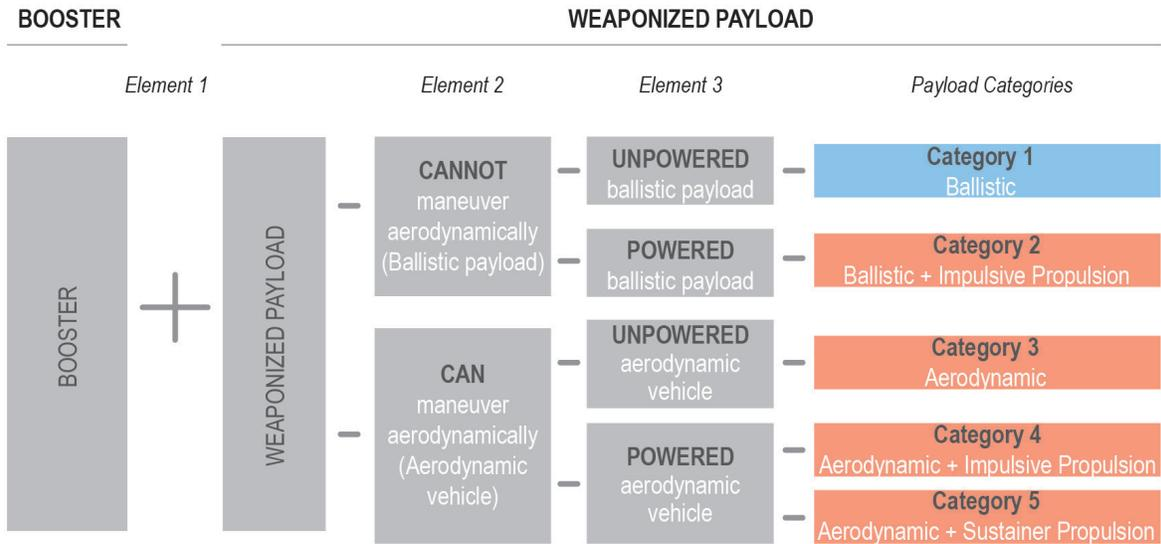
**Figure 5: Combinations of fundamental missile system elements.**
