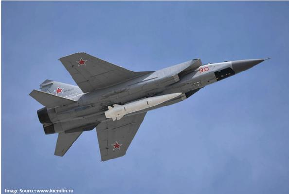
**Figure 4: Russian Kinzhal medium-range ALBM on Mig-31 Interceptor.** (Capable of maneuvering aerodynamically after boost.)
