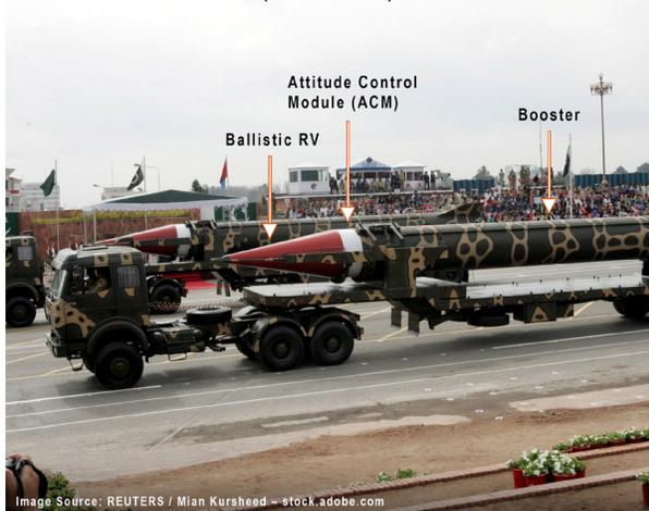
**Figure 11: Example Category 2 missile system with an ACM payload.**
