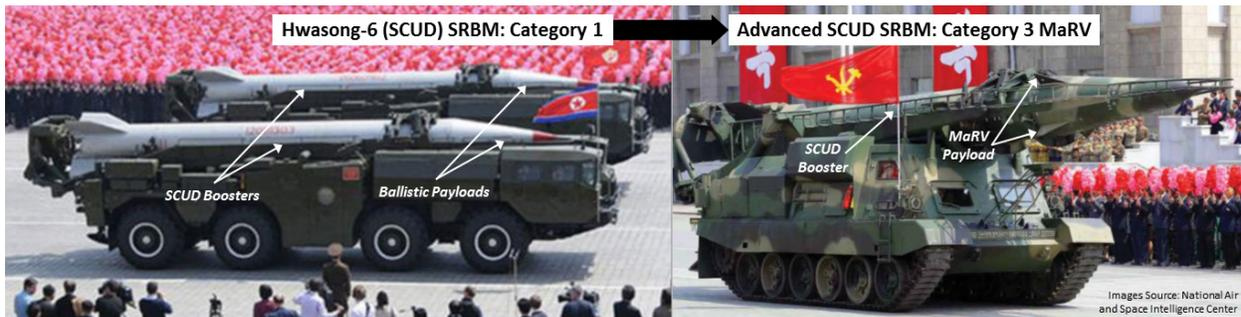
**Figure 16: Example: Transition of ballistic missile boosters to Category 3 (MaRV) payloads (North Korean SCUD booster).**
