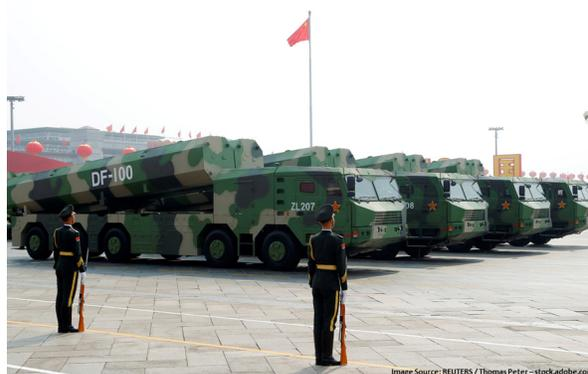
**Figure 20: Example: Chinese medium-range DF-100 cruise missile dual-canister launchers (MRM5: Supersonic).**
