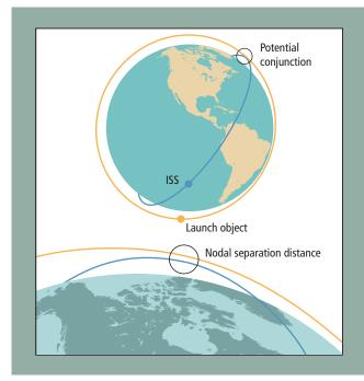
An illustration of the nodal separation distance between the orbit of the International Space Station and the orbit of a spent upper stage.
