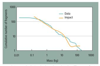
A cumulative mass distribution plot shows the total number of fragments of a given mass and larger. The more energetic the event, the steeper its mass distribution slope. Therefore a greater fraction of the mass is in smaller fragments, where the debris is more pulverized.
