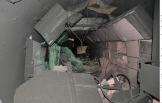
at nearly 7 kilometers per second, a record for that size object. The resulting soft catch foam, which lined the test chamber, and the debris the foam contained, filled more than 40 shipping pallets. Debris processing is ongoing.
