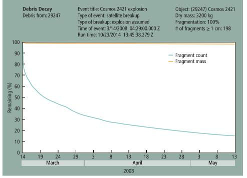
Debris-decay plots such as this show the percentage of fragments and total fragment mass remaining in orbit over time.
