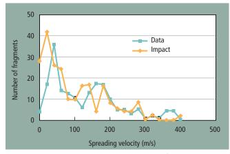
Spreading speed distributions show how the magnitudes of the changes in velocity given the fragments by the event are distributed. The analysis of the Landsat 3 Delta II upper stage explosion, as seen in the mass, velocity distribution, and AMR distribution plots (top figures and this one) of its trackable debris, is a good example of how default assumptions within IMPACT can produce close approximations to event characteristics.
