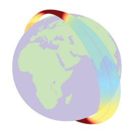
The Debris Torus provides a more useful sense of the concentration of space debris. This image shows a model of the Chinese Fengyun-1C breakup, 14 days after collision. Highly concentrated regions near the poles are shown as solid red sections, while less concentrated regions near the equator are shown as transparent and blue.
