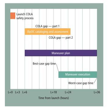
Collision-avoidance assessments for launches have a limited shelf life. The accuracy of predicted positions for launched objects quickly degrades. This leads to a dangerous gap in situational awareness until the Space Surveillance Network can register and track the launched items.
