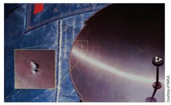
A small piece of space debris traveling at 17,000 miles per hour carries a lot of energy. This photo depicts damage to the Hubble telescope caused by debris.
