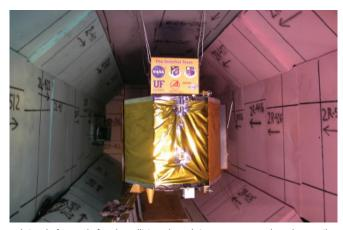
DebriSat before and after the collision. The DebrisLV test was conducted on April 1, 2014, followed by the DebriSat test on April 15. Both tests used an aluminum and nylon cylindrical projectile with a mass of slightly less than 600 grams and propelled
