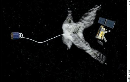
A conceptual rendering of a capture and deorbit device for space debris cleanup.
