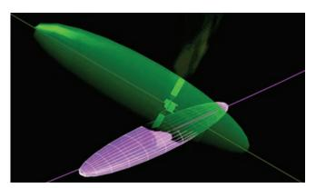
To help predict possible collisions, mission operators rely on visualizations such as this, which shows the intersection of covariance ellipsoids for two orbiting objects (note: the satellites depicted are not to scale within the ellipsoids).
