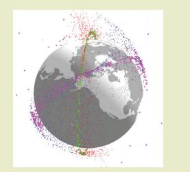
This image compares the cataloged debris from Iridium 33 (green) and Cosmos 2251 (purple) for sizes approximately 10 centimeters or larger. Overlaid in red and blue are Aerospace models of the 1 centimeter and larger debris that is untrackable.
