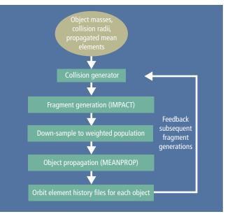
These flowcharts illustrate the ADEPT process for generating future debris population models. The first shows the high-level flow of the overall simulation, and the
