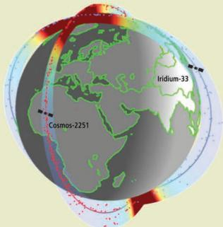
The debris Torus was used to model the Iridium-Cosmos collision of 2009. Areas of higher risk are easy to identify.
