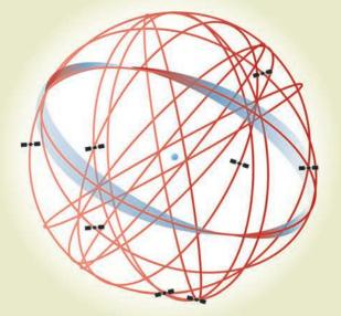
A Walker constellation that lies at the same orbital altitude as a debris field may have multiple crossings. The precise timing of these penetration intervals can be quickly calculated using Torus data and fed to operators, allowing them to make maneuver decisions. The Torus visualization makes it easier to grasp the nature of the problem.(Note that Earth has been scaled down to enable viewing of both sides of the orbit.)
