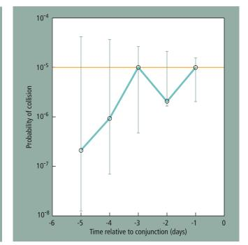
Confidence intervals on probability estimates are useful tools for satellite operators. In this graph, the circles indicate the probability of collision predicted for Day 0 using the best information available, with the error bar indicating the range of possible values. The yellow line indicates a user-selected threshold for action. The satellite operator can use this to understand the quality of the prediction and make a better decision by comparing it to an action threshold.
