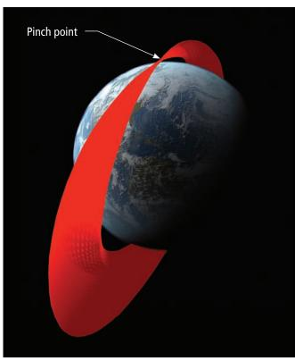
As the mechanics of orbital motion come into play, the cloud of fragments—the debris—spreads around the orbit close to the plane of the parent orbit. Eventually, all of the debris will return to the point of the collision, because that point is common to the orbits of all the debris. This is called the pinch point.
