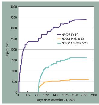
These plots show how the amount of cataloged debris from three fragmentation events expanded over time.
