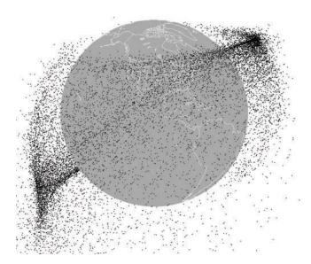
The standard method of representing debris as individual dots on a computer screen gives a false impression of the extent of the debris hazard.
