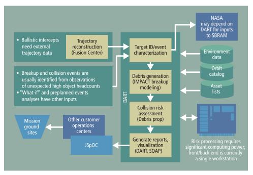
The DART process uses Aerospace's IMPACT model to create a statistical cloud of breakup debris that includes fragments down to 1 centimeter. The data can then be used to model a variety of breakup events and quantify the risks to active satellites. The SBRAM refers to NASA's satellite breakup risk assessment model.
