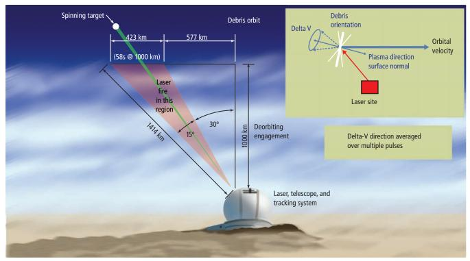
A laser broom concept for space debris removal and cleanup.
