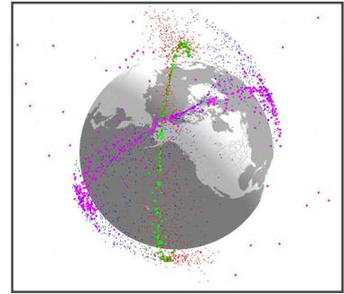
This image models the debris from the 2009 collision of the Iridium-33 (green) and Cosmos2251 (purple) satellites. Overlaid in red and blue are Aerospace models of estimated untrackable debris.
