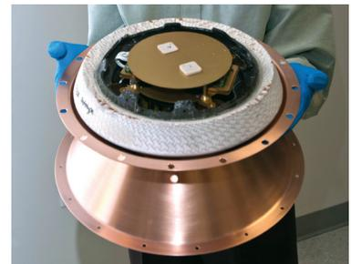
The first Reentry Breakup Recorder (REBR) successfully recorded data as it plunged through the atmosphere aboard a disintegrating Japanese HTV-2 spacecraft. Data was transmitted to ground systems via the Iridium satellite system.
